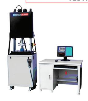
Used to determine the durability of materials such as metals, plastics, rubber and complex stuff.
